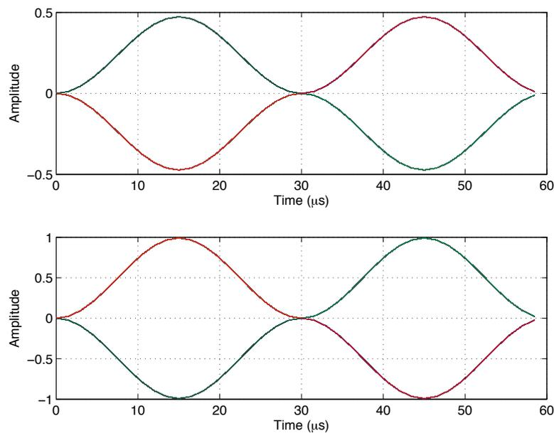
**Figure:** Eye diagram for received signal;  $T_s = 30\mu\text{s}$ . No distortion: “the eye is fully open”.
