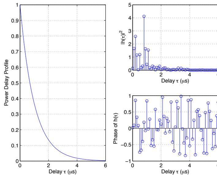
**Figure:** Power Delay Profile and Channel Impulse Response; the power delay profile (left) equals  $\Psi_h(\tau) = \exp(-\tau/T_h)$  with  $T_h = 1\mu\text{s}$ ; one possible realization of magnitude and phase of impulse response (left).
