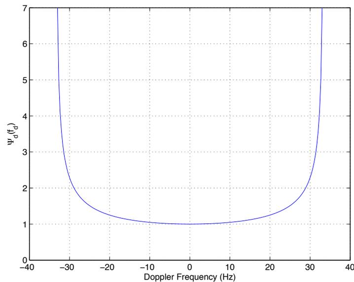
**Figure:** Doppler Spread Function for Isotropic Scatterer; velocity  $v = 10\text{m/s}$ ,  $f_c = 1\text{GHz}$ , maximum Doppler frequency  $f_d \approx 33\text{Hz}$ . First zero at  $\Delta t \approx 0.4/f_d$ .
