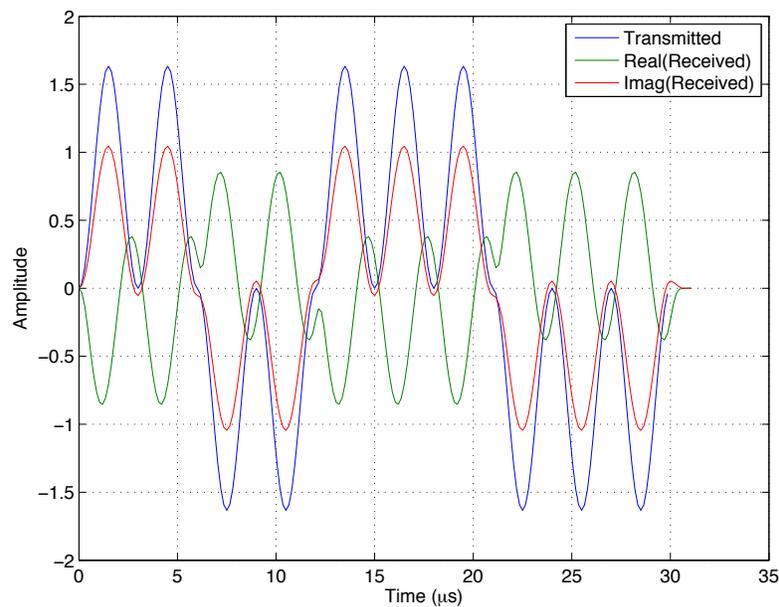
**Figure:** Transmitted and received signal;  $T_s = 3\mu\text{s}$ . Some distortion is visible near the symbol boundaries.
