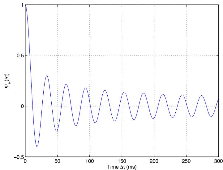
**Figure:** Time-Coherence Function for Isotropic Scatterer; velocity  $v = 10\text{m/s}$ ,  $f_c = 1\text{GHz}$ , maximum Doppler frequency  $f_d \approx 33\text{Hz}$ . First zero at  $\Delta t \approx 0.4/f_d$ .
