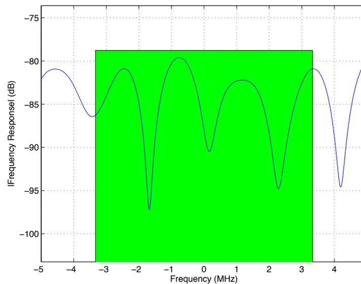
**Figure:** Frequency Response of Channel and bandwidth of signal;  $T_s = 0.3\mu s$ , Bandwidth  $\approx 6$  MHz; the channel's frequency response varies significantly over the bandwidth of the channel.
