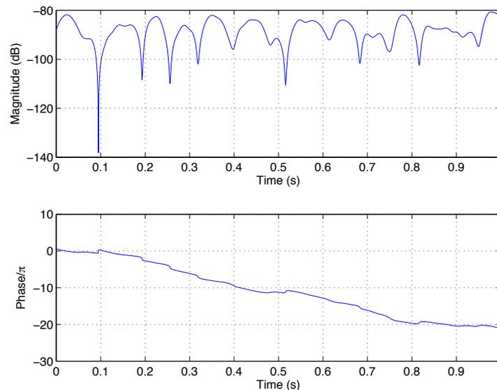
**Figure:** Response of channel to sinusoidal input signal; base-band equivalent input signal  $s(t) = 1$ , velocity  $v = 10\text{m/s}$ ,  $f_c = 1\text{GHz}$ , maximum Doppler frequency  $\approx 33\text{Hz}$ .
