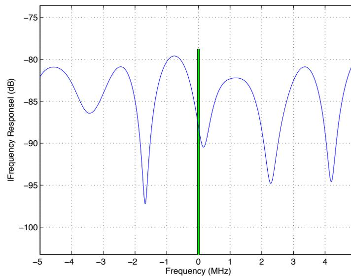
**Figure:** Frequency Response of Channel and bandwidth of signal;  $T_s = 30\mu s$ , Bandwidth  $\approx 60$  KHz; the channel's frequency response is approximately constant over the bandwidth of the signal.
