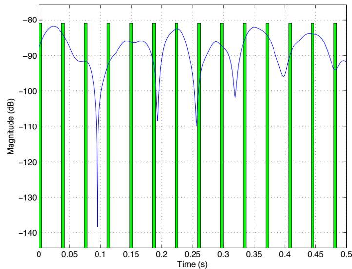
**Figure:** Time varying channel response and TDMA time-slots; time-slot duration 4.6ms, 8 TDMA users, velocity  $v = 10\text{m/s}$ ,  $f_c = 1\text{GHz}$ , maximum Doppler frequency  $\approx 33\text{Hz}$ .
