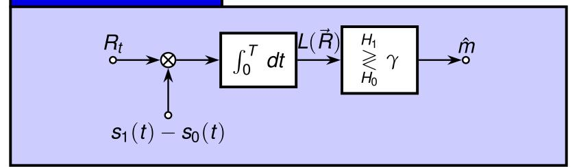
The two correlators can be combined into a single correlator for an even simpler frontend.
