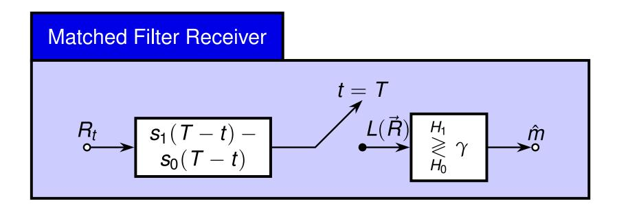
The filter with impulse response  $h(t) = s_1(T-t) - s_0(T-t)$  is called the matched filter for  $s_1(t) - s_0(t)$ .
