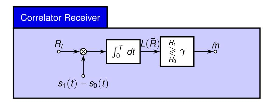
► The two correlators can be combined into a single correlator for an even simpler frontend.
