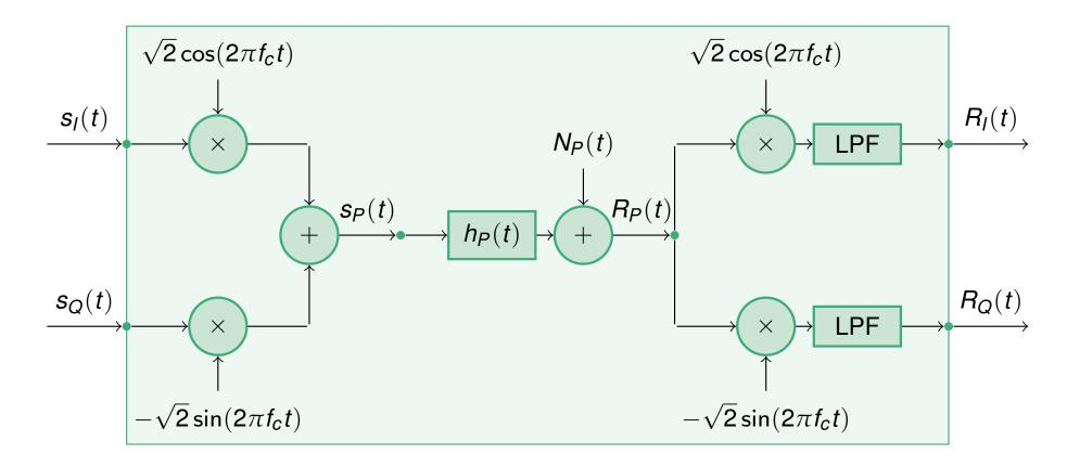
Complete pass-band system with channel (filter) and passband noise.
