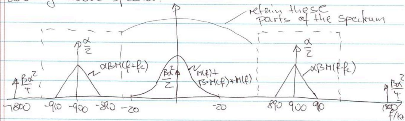
b) The bandpass filter must pass frequencies between 890 and 910 kHz!
