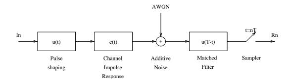
The objective of this problem is to determine the parameters of the equivalent tapped delay-line model between the input sequence  $I_n$  and the output sequence  $R_n$ . A generic block diagram for a tapped delay-line model is given below.
